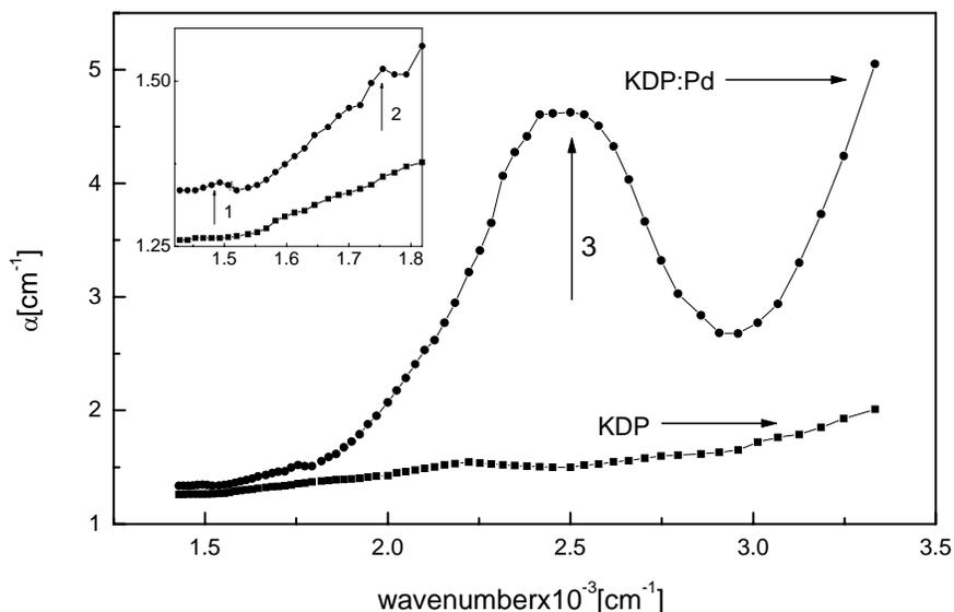
Fig. 1. The absorption spectra of the KDP and KDP:Pd crystals in the  $13300 \div 35000 \text{ cm}^{-1}$  spectral range. The insert shows only the low energy spectral range in the same units.
