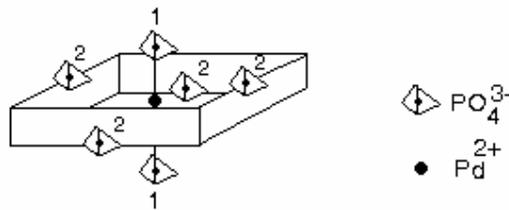
Fig. 2. The presumed configuration of the Pd<sup>2+</sup>-complex in KDP:Pd crystal. For clarity the protons have been omitted.
