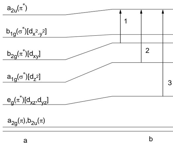
Fig. 3. Molecular orbital energy level scheme; **a**- for pure square planar transition metal complex in which the ligands themselves have a  $\pi$ -orbital system and **b**- presumed scheme for pseudo-square planar  $Pd^{2+}$ -complex in KDP:Pd crystal.
