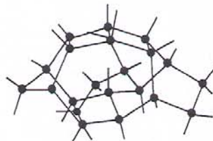
Fig. 4 A dangling bond in a continuously interconnected tetrahedrally bonded random network (Si, Ge).
