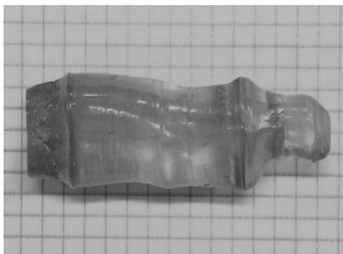
Fig. 1. As- grown single crystal of \text{Li}_6\text{Gd}_{(1-x)}\text{Ce}_x(\text{BO}_3)_3 (a division=5 mm).
