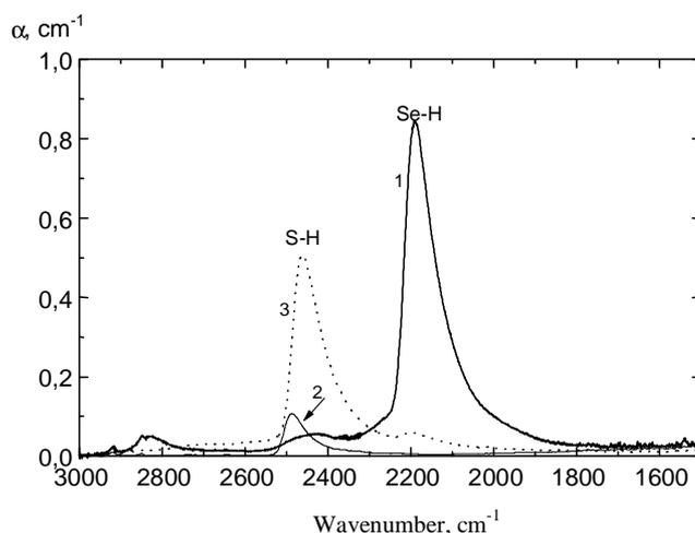
Fig. 5. A hydrogen transfer from Se to S in the mixed  $\text{As}_2\text{S}_3$ - $\text{As}_2\text{Se}_3$  glasses. 1, 2, 3 - absorption spectra of  $\text{As}_2\text{Se}_3$ ,  $\text{As}_2\text{S}_3$  and  $(\text{As}_2\text{Se}_3)_{0.95}(\text{As}_2\text{S}_3)_{0.05}$  glasses, respectively.
