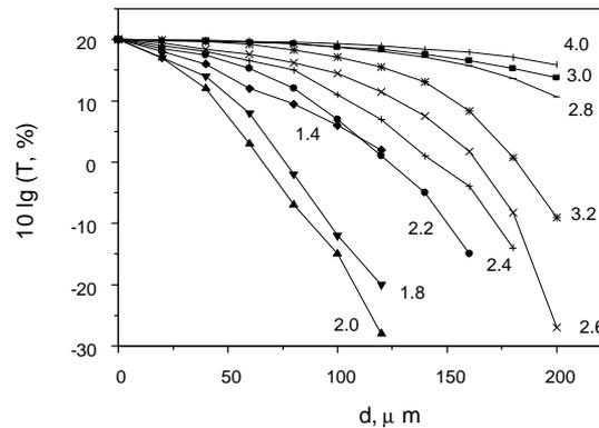
Fig. 2. Optical transmission characteristics vs. displacement amplitude for different microbend periods.  $\Lambda = 1.4-4.0$  m. The light source was a He-Ne laser coupled through a 90x microobjective.
