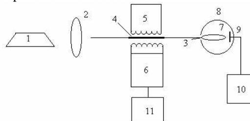
Fig. 1. Experimental set-up: 1 - light source; 2 - microobjective; 3 - optical fibre; 4 - glycerine; 5 - deformer; 6 - piezoelectric transducer; 7 - the bent segment of the fiber; 8 - integrating sphere; 9 - photodiode; 10 - lock-in amplifier; 11 - generator.
