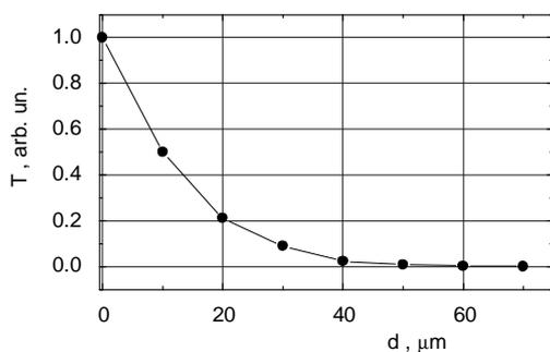
Fig. 3. Optical transmission characteristic for microbending period 1.8 mm.
