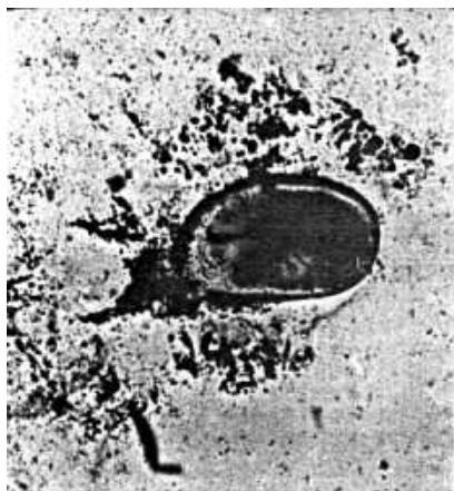
Fig. 3. Images of the film \text{Se}_{42}\text{S}_{58} in the region of impact of a simple laser pulse (ruby) of energy 980 mJ immediately after impact.
