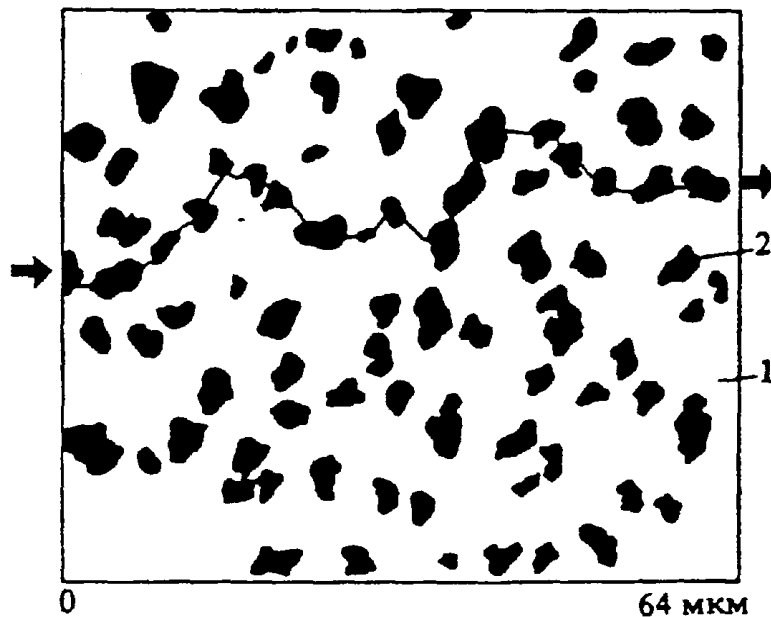
Fig. 2. Distribution of elements over the sample cross-section, obtained by means of X-ray microanalysis (reproduced from [1]). (1) Selenium and (2) HTSC. The solid, broken line showing the path of the through current represents a set of superconducting Se channels connecting adjacent HTSC globules.
