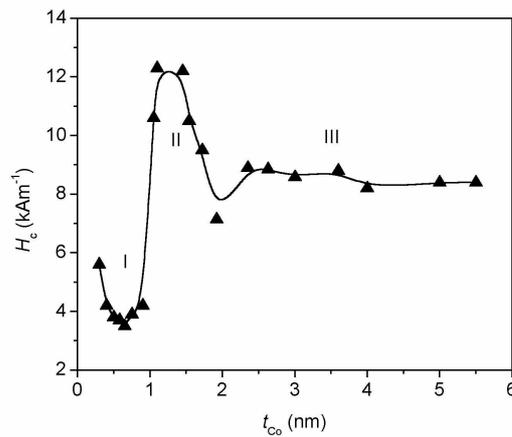
Fig. 2. Coercive field  $H_c$  as a function of  $t_{Co}$  for a series of Co/Pt multilayers with  $t_{Pt} = 1$  nm.
