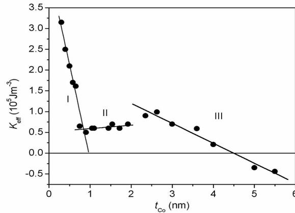
Fig. 1. Magnetic anisotropy constant  $K_{eff}$  as a function of nominal thickness of Co layer ( $t_{Co}$ ) for a series of Co/Pt multilayers with  $t_{Pt} = 1$  nm.
