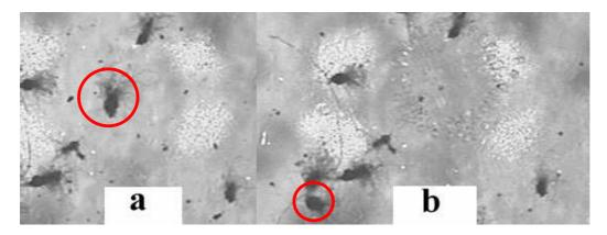
Fig. 4. Spores of *Chaetomium sp.*(a) have been slowly displaced by laser cleaning (b).
