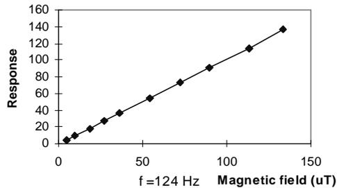
Fig. 1. The Envirometer response on the 200  $\mu\text{T}$  scale with magnetic field variation.
