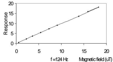
Fig. 2. The Envirometer response on the 20  $\mu\text{T}$  scale with magnetic field variation.
