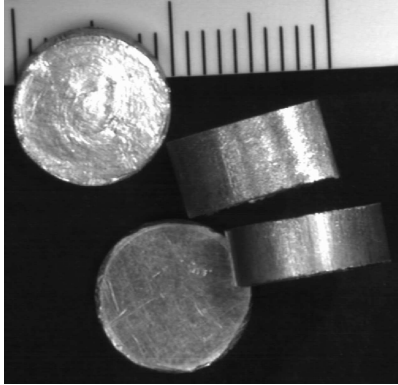
Fig. 5. Hot pressed discs from \text{Fe}_{77}\text{Al}_{2.14}\text{Ga}_{0.86}\text{P}_{8.4}\text{C}_5\text{B}_4\text{Si}_{2.6} amorphous alloy powder.
