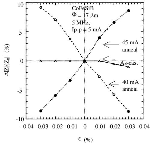
Fig. 4. Z vs.  $\epsilon$  characteristics for Co-based 17  $\mu$ m wires.
