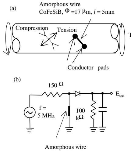
Fig. 7. Torque measuring system.
