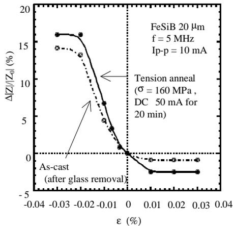
Fig. 5. Z vs.  $\epsilon$  characteristics for Fe-based 20  $\mu$ m wires.
