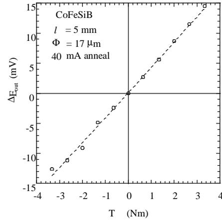
Fig. 8. Typical output characteristics of the impedance gauge sensor for torque detection.
