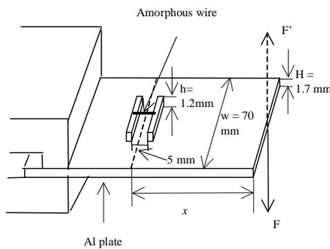
Fig. 1 Experimental system for impedance gauge characteristics.
