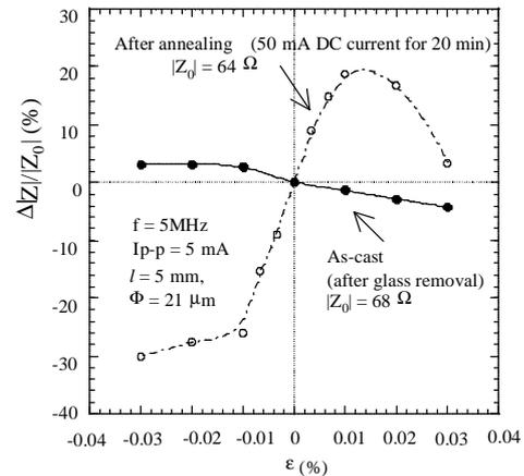
Fig.2.  $Z$  vs.  $\epsilon$  characteristics for Co-based 21  $\mu\text{m}$  wires.
