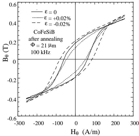
Fig.3. Change in  $B_0H_0$  loops with a strain for Co-based wires.
