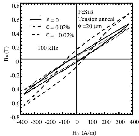
Fig. 6.  $B_0H_0$  loops for Fe-based wires.
