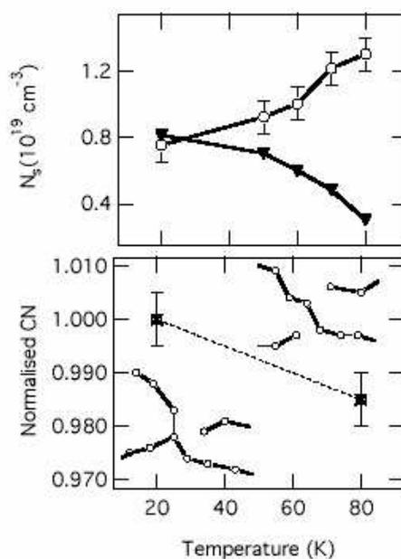
Fig. 2. Complementary temperature dependence of concentration of the two types of photo-induced ESR centres (top) is accompanied by a decrease in the average coordination number (bottom) suggesting that three - fold coordinated defects are decomposed into a normally
