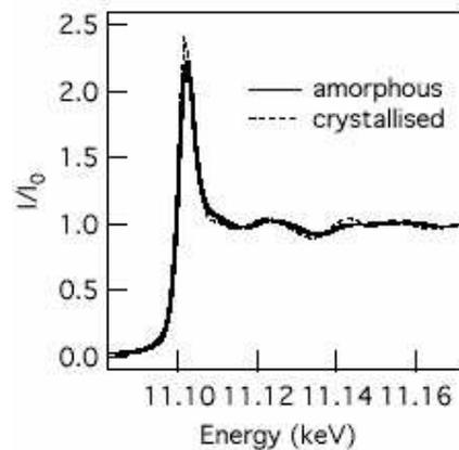
Fig. 5. XANES spectra of amorphous and crystallized GST films.
