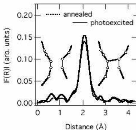
Fig. 1. FT EXAFS spectra of annealed and photoexcited a-Se film measured at 30 K. An increase in the peak magnitude is caused by the cross-linking of the neighbouring chains.
