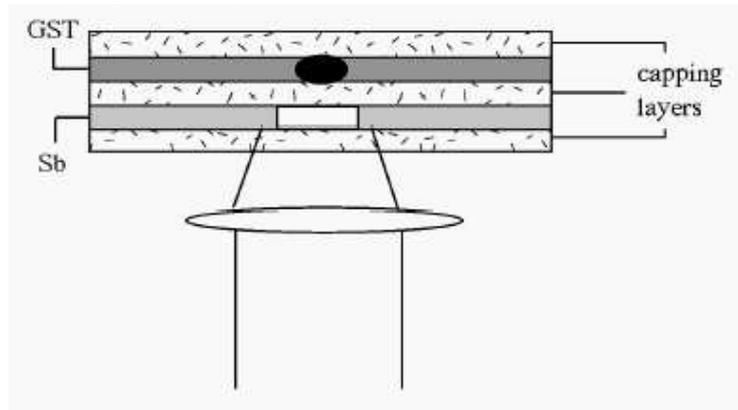
Fig. 4. A schematic presentation of transmission Super-RENS.
