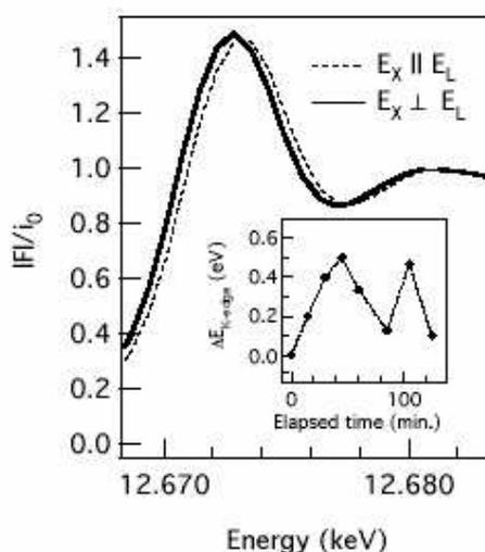
Fig. 3. K-edge XANES spectra of s-Se film irradiated by linearly polarized light with the polarization plane oriented parallel and perpendicular to the polarisation plane of the probing x-ray beam. The insert shows a reversible shift of the edge upon rotation of the polarization
