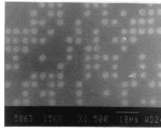
Fig. 2. Scanning electron micrograph of a computer generated holographic pattern produced by InO<sub>x</sub> microprinting on glass.
