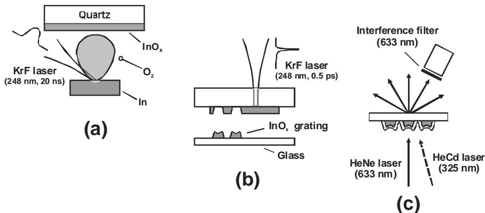
Fig. 1. Outline of  $\text{InO}_x$  grating development and testing (a) pulsed laser deposition of the  $\text{InO}_x$  targets, (b)  $\text{InO}_x$  grating microprinting, and (c) optical diffraction and grating activation.
