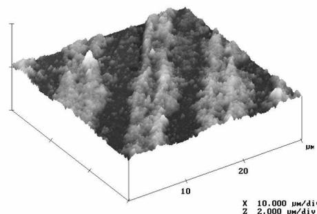
Fig. 3. Atomic force microscope (AFM) image of a small portion of a typical InO<sub>x</sub> grating.
