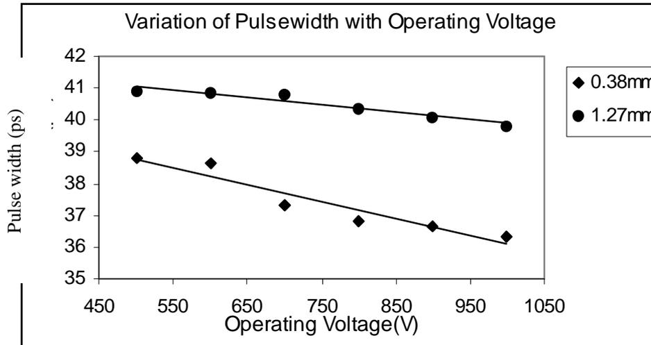
Fig. 3. Variation in output pulse width with operating Voltage and width of Dye cell.
