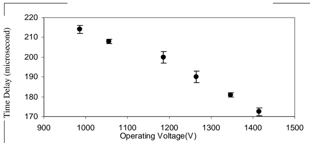
Fig. 1. Variation of time delay with operating voltage.
