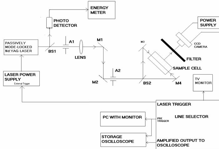
Fig. 2. Two photon fluorescence experimental setup.
