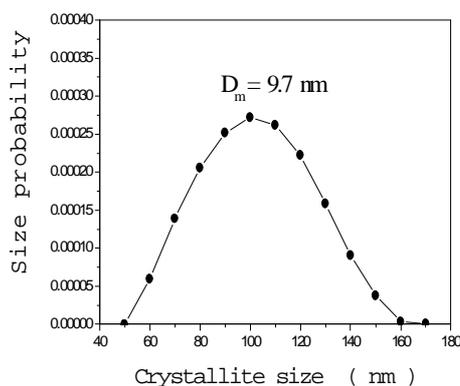
Fig. 2. The crystallite size distribution as a function of the effective crystallite size along the perpendicular direction to the (111) planes (after Aldea and Indrea, 1990).
