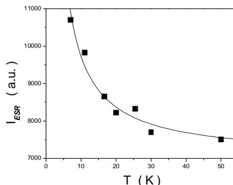
Fig. 4. Temperature dependence of the ESR. The solid line corresponds to the Curie law giving the best fit to the data.
