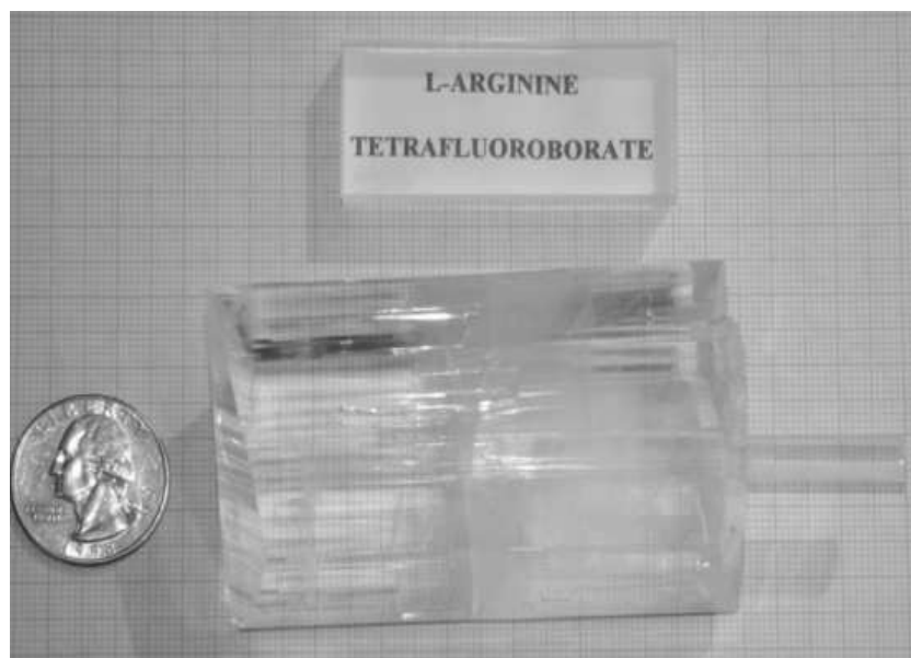
Fig. 2. A photograph of L-HFB crystal grown at Alabama A&M University.
