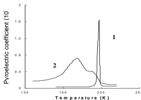
Fig. 3. The pyroelectric coefficient temperature dependence. Curve 1 - TlInS<sub>2</sub> crystal; Curve 2 - TlInS<sub>2</sub><Fe> crystal.
