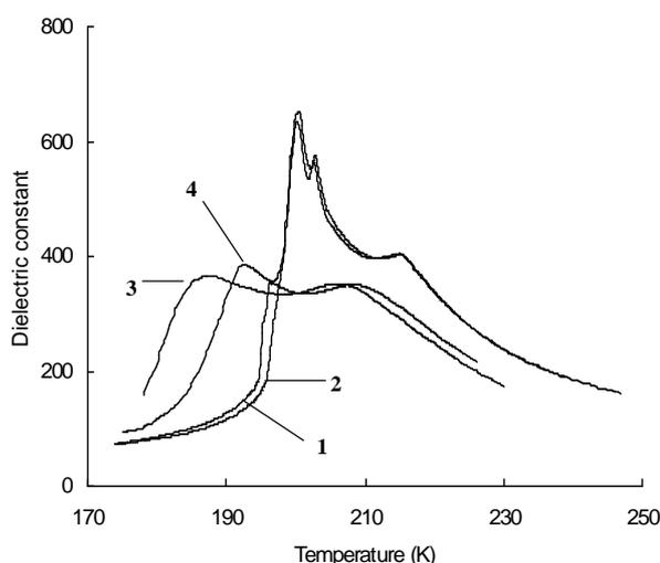
Fig. 1. The dielectric constant  $\epsilon(T)$  temperature dependencies. Curves 1, 2 - the dependences  $\epsilon(T)$  of  $\text{TlInS}_2$  crystal (1 - cooling; 2 - heating); Curves 3, 4 - the dependences  $\epsilon(T)$  of  $\text{TlInS}_2\langle\text{Cr}\rangle$  crystal (3 - cooling; 4 - heating).
