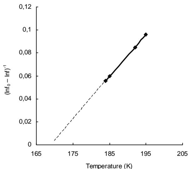
Fig. 4. The dependence  $(\ln f_0 - \ln f)^{-1}$  from  $T_m$  for  $\text{TIInS}_2\langle\text{Cr}\rangle$ , illustrating the validity of the Vogel-Fulcher law.
