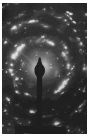
Fig. 5. SAED pattern of a PZT layer observed in plan view, subjected only at a pyrolysis step (450 °C, 2 min), without drying. Besides the quasi-amorphous ring of an intermediate fluoritic phase and the very weak ring associated to TiO 2 , some strong spots of cubic TiO are present.
