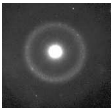
Fig. 3. SAED pattern showing the vanishing of cubic TiO rings and the presence of a perovskitic or intermediate phase with a weak crystallization.
