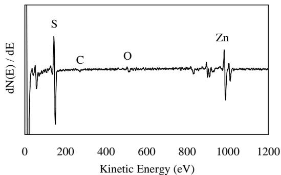
Fig. 7. AES spectrum for the film deposited with Rochelle salt (sample (b-2)).
