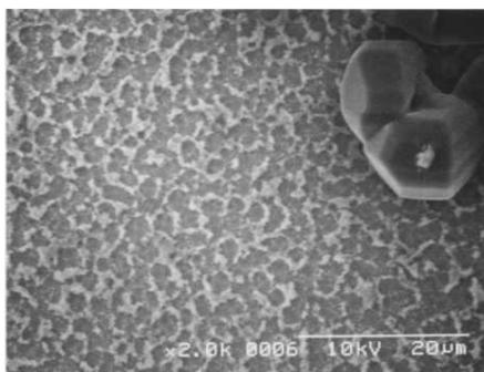
Fig. 6. SEM picture of the film deposited with Rochelle salt (sample (b-2)).
