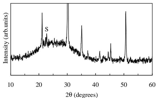
Fig. 8. XRD pattern for the film deposited with Rochelle salt (sample (b-2)).
