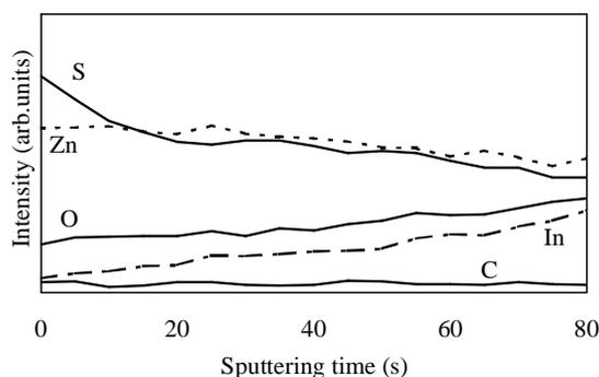
Fig. 4. AES depth profile for the film deposited without Rochelle salt.
