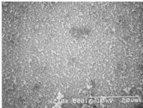
Fig. 2. SEM picture of the film deposited without Rochelle salt.
