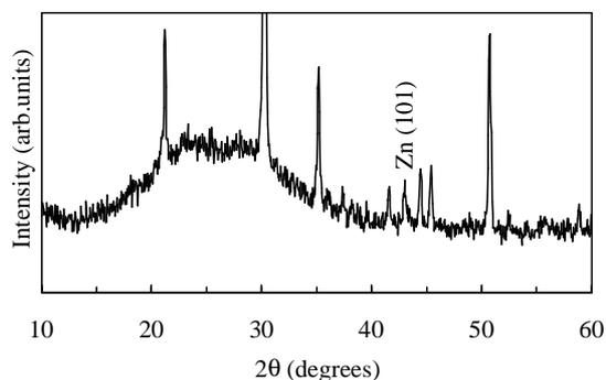
Fig. 5. XRD pattern for the film deposited without Rochelle salt.
