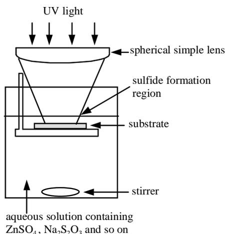
Fig. 1. Sketch of the apparatus for PCD.
