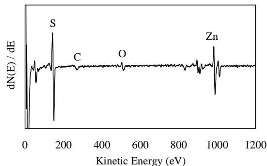
Fig. 3. AES spectrum for the film deposited without Rochelle salt.
