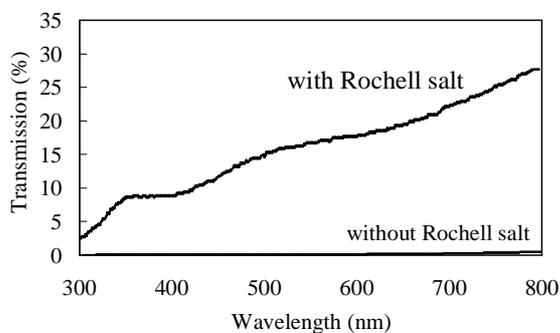
Fig. 9. Transmission spectra for the films deposited with and without Rochelle salt.
