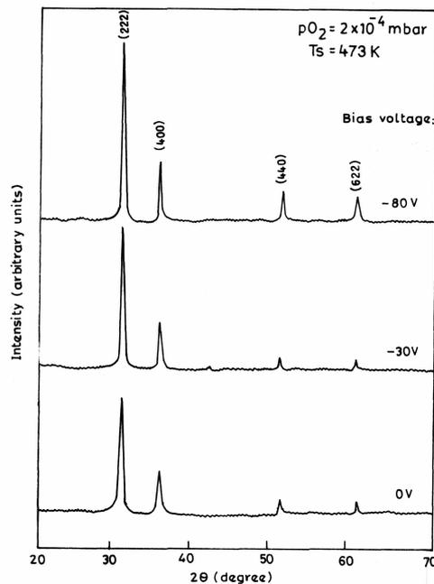
Fig. 3. X-ray diffraction patterns of  $\text{In}_2\text{O}_3$  films formed at  $473$  K under various substrate bias voltage.
