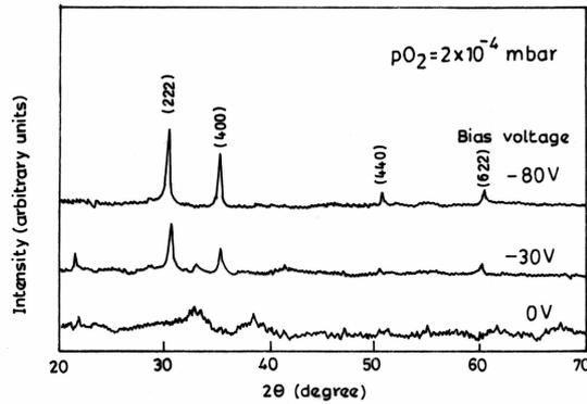
Fig. 1. X-ray diffraction patterns of  $\text{In}_2\text{O}_3$  films formed at  $303$  K under various substrate bias.
