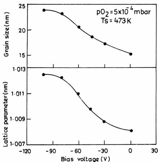
Fig. 4. Variation of lattice parameter and grain size on the substrate bias of  $\text{In}_2\text{O}_3$  films formed at 473 K.
