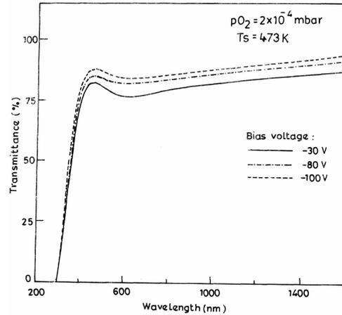
Fig. 6. Optical transmittance spectra of  $\text{In}_2\text{O}_3$  films formed at 473 K at different substrate bias voltages.
