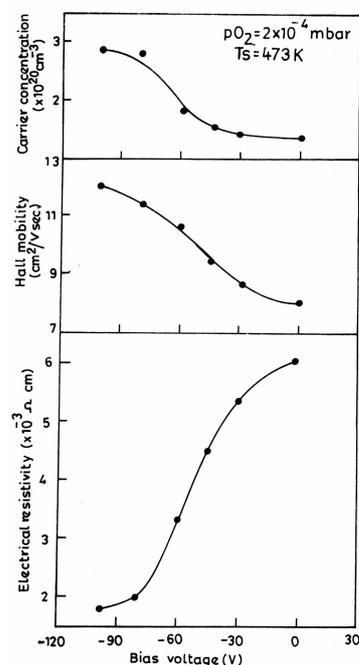
Fig. 5. Dependence of electrical resistivity, Hall mobility and carrier concentration of  $\text{In}_2\text{O}_3$  films deposited at 473 K on the substrate bias voltage.
