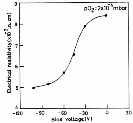
Fig. 2. Dependence of electrical resistivity of  $\text{In}_2\text{O}_3$  films formed at  $303$  K on the substrate bias voltage.
