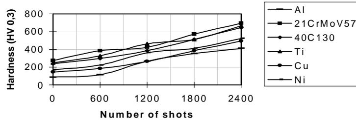
Fig. 3. Surface target hardness vs. number of laser shots.
