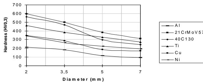
Fig. 4. Surface target hardness vs. laser spot diameter.
