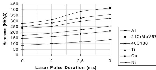
Fig. 2. Surface target hardness vs. laser pulse duration.
