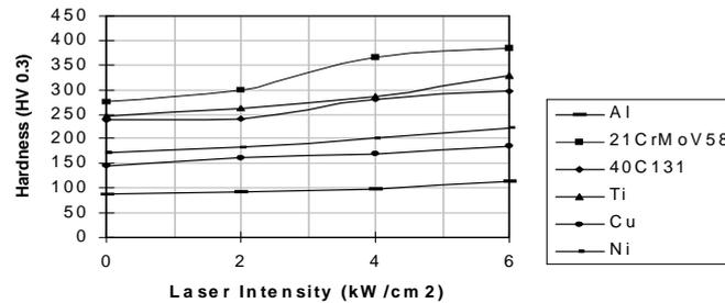
Fig. 1. Surface target hardness vs. laser intensity.
