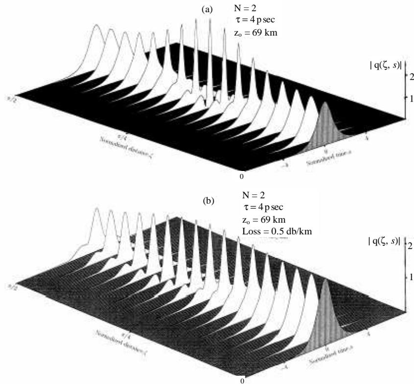
Fig. 1. Propagation of the single second order soliton. (a) without the loss, (b) with the loss.
