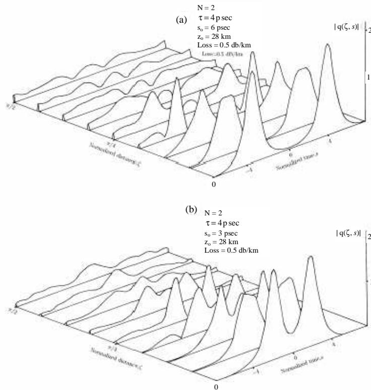
Fig. 3. Propagation of the two second order soliton under the effect of the optical fiber loss. (a) Pulse separation 12 psec, (b) Pulse separation 6 psec.
