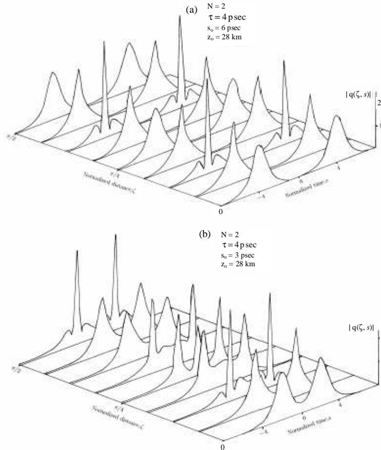
Fig. 2. Propagation of the two second order soliton through lossless optical fiber. (a) Pulse separation 12 psec, (b) Pulse separation 6 psec.
