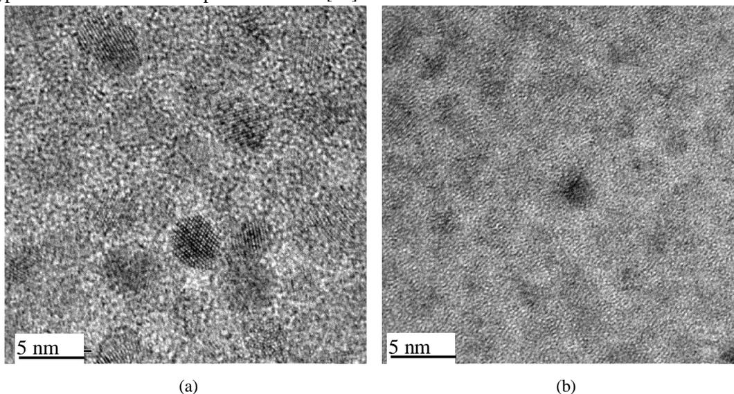
Fig. 1. Bright-field electron micrograph of the as-cast  $\text{Nd}_{50}\text{Fe}_{40}\text{Al}_{10}$  melt-spun ribbons: (a) 25  $\mu\text{m}$ , and (b) 120  $\mu\text{m}$  thickness.
