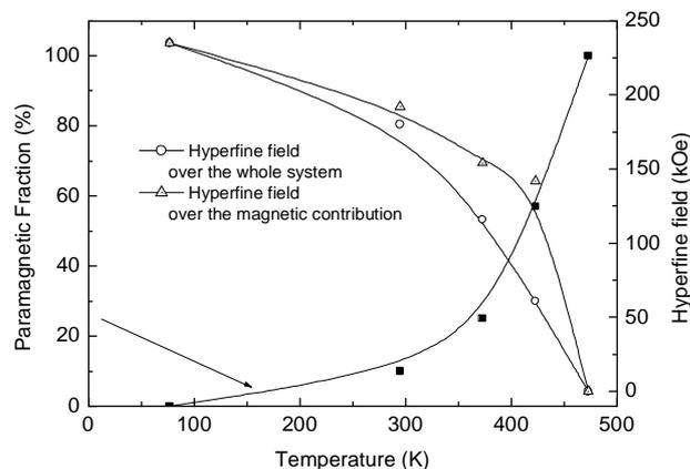
Fig. 3. Hyperfine fields and the evolution of the paramagnetic fraction vs. temperature as resulted from Mössbauer data.
