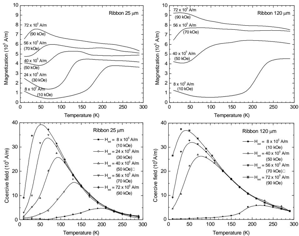
Fig. 2. Magnetization and coercive field vs. temperature for amorphous melt-spun ribbons  $\text{Nd}_{50}\text{Fe}_{40}\text{Al}_{10}$ .
