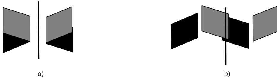
Fig. 2. a) shows the position of the wings in the object plane, (the wings are superposed); b) shows the position of the wings in the laser focal plane situated at 150\ \mu\text{m} (the wings are displaced one from another with a distance between wings and a quarter of wing).
