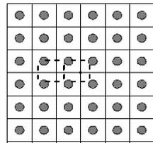
Fig. 3. Square lattice structure. Grey circles represent the inclusions distributed in the host media.
