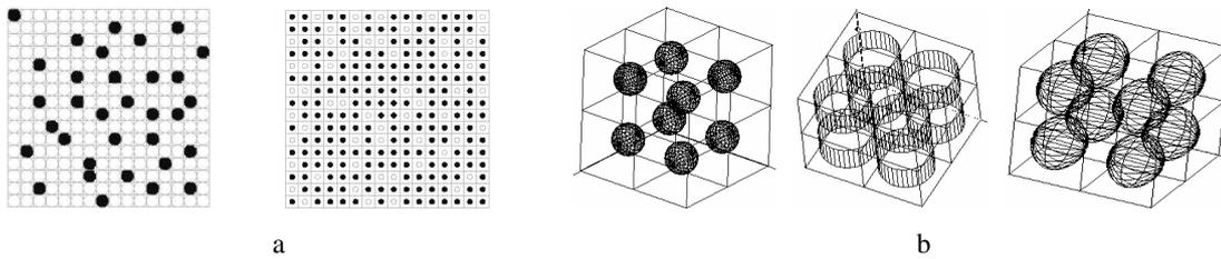
Fig. 2. Structures with: a – cylindrical inclusions of different size for the same filling factor; b – spherical, elliptical and cylindrical inclusions.
