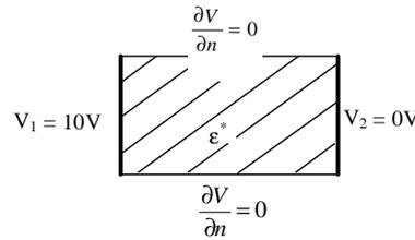
Fig. 4. Boundary conditions assigned to the model.
