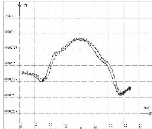
Fig. 6. Magnetoresistance of permalloy thin film, 100 nm, deposited by RF sputtering,  $V_i = 10 \text{ mV}$ .
