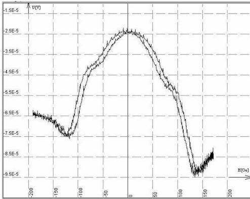
Fig. 5. Magnetoresistance of evaporated permalloy thin film, 100 nm,  $V_i=10\text{mV}$ .
