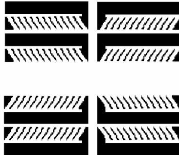
Fig. 2. Detail of mask for deposition of gold strips, x100.
