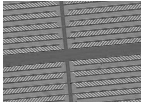
Fig. 4. Detail of magnetoresistive microsensors, x100.
