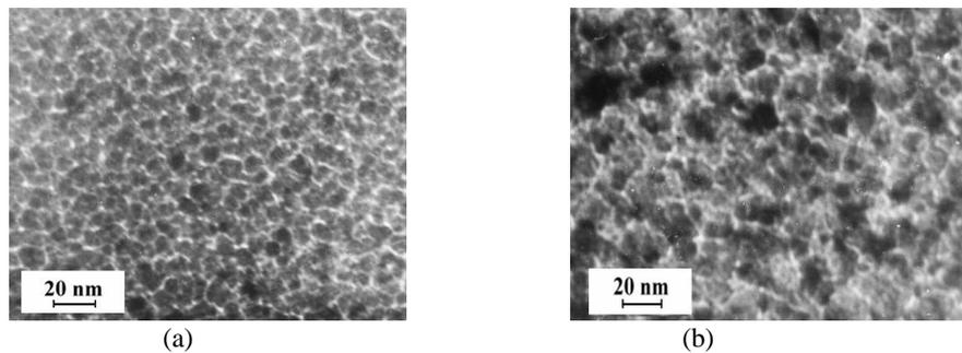
Fig. 2. TEM micrographs of  $[\text{FeCoB}(12\text{nm})/\text{SiO}_2(2\text{nm})] \times 5$  thin films: in as-deposited state (a); after annealing at  $400^\circ\text{C}$ .
