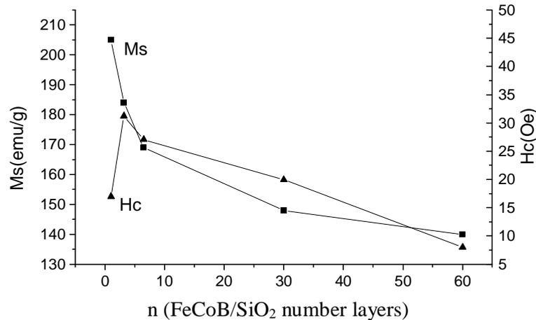
Fig. 1. Dependence of the magnetization and coercive field on the FeCoB/SiO<sub>2</sub> number layers (n).
