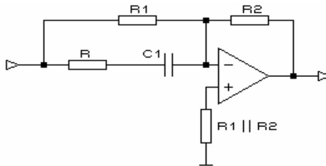
Fig. 1. Common PD controller.
