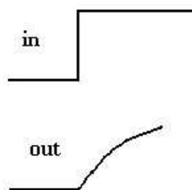
Fig. 3. Output of a PID controller to a step input.
