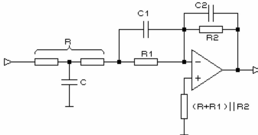
Fig. 4. Structure used for the thermopile signal accelerator / averager circuit.
