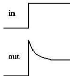
Fig. 2. Output of a PD controller to a step input.
