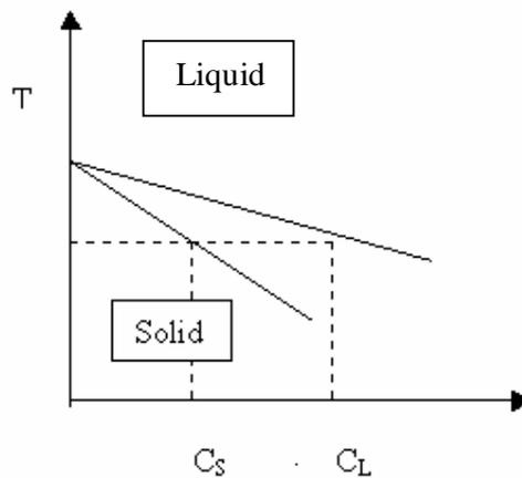
Fig. 3. Phase diagram for a binary system.
