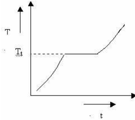
Fig. 2. Heating curve for crystallization from melt.
