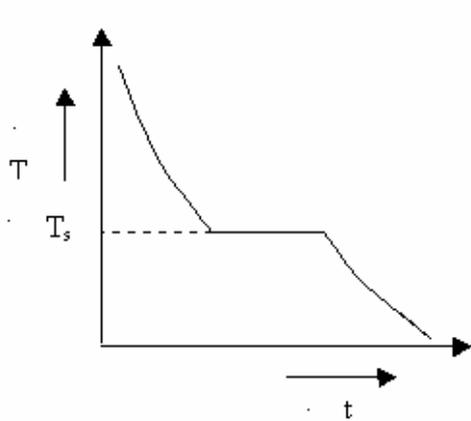
Fig. 1. Cooling curve for crystallization from melt.
