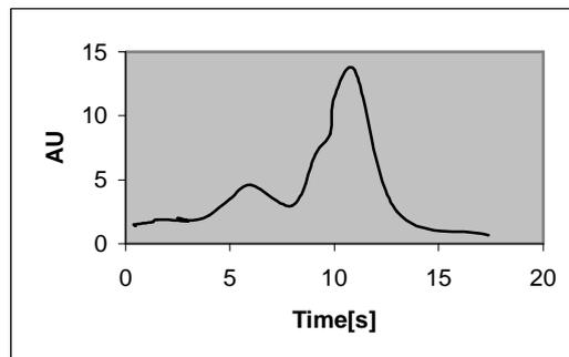
Fig. 6. Brightness curve of LiF: Mg, Ti (chips) detectors after thermal treatment.
