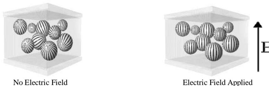
Fig. 1. Change of the orientation of LC molecules in an electric field [1].
