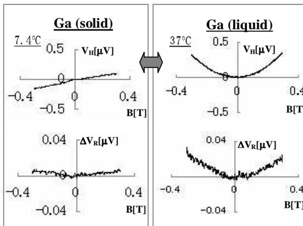
Fig. 11. Hall effect and magnetoresistance effect for Ga (in liquid and solid state).
