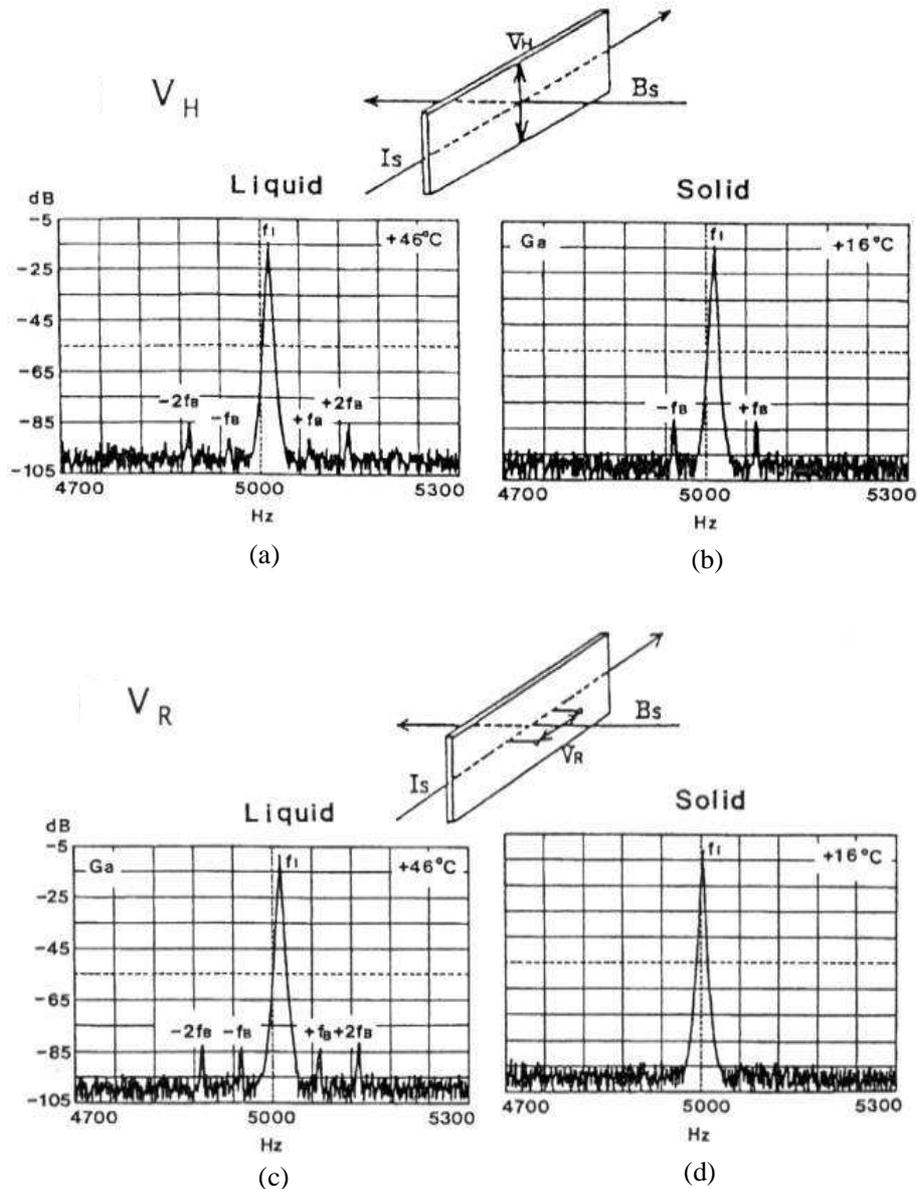
Fig. 9. Spectra of (a), (b) Hall voltage by means of the two-frequency ac method and (c), (d) variation of voltage by means of the four point probe method, for Ga at  $46^\circ\text{C}$  and solid Ga at  $16^\circ\text{C}$ , in the high frequency region for a 5 kHz sample current and 0 kHz, 0.23 T magnetic field, respectively.
