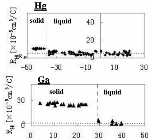
Fig. 12. Temperature dependence of Hall coefficient in Ga and Hg.
