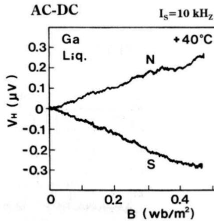
Fig. 8. Hall signals for liquid Ga at 40 °C through ac-dc method at 7kHz ac current.
