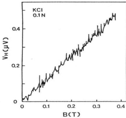
Fig. 2. Hall voltage vs. magnetic field measured by the two - frequency ac method.
