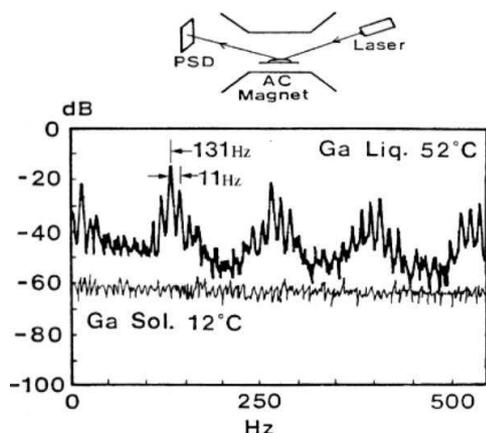
Fig. 5. The spectrum measured with the two-frequency ac method consisting of 60 Hz of ac-B and 71 Hz of ac-I shows surface movements of the liquid Ga sample at 52 °C accompanied by many higher harmonics including pseudo signals of 11 and 131 Hz. These features cannot be seen for the solid state Ga at 12 °C.
