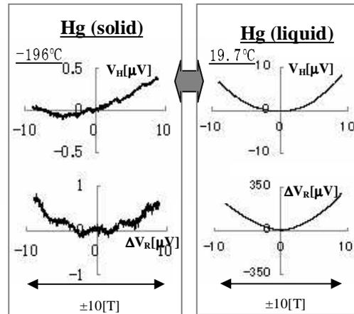
Fig. 13. Hall effect and magnetoresistance effect for Hg (in liquid and solid state) at high magnetic field vertical units are different.
