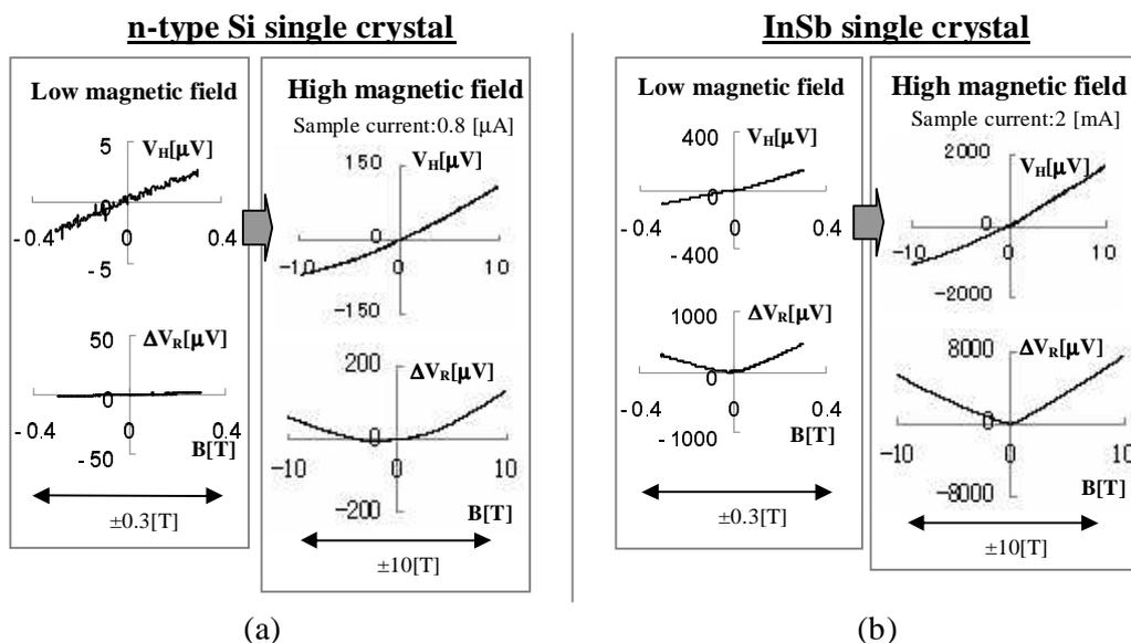
Fig. 14. Hall and magnetoresistance effect in InSb and n-type Si single crystal.
