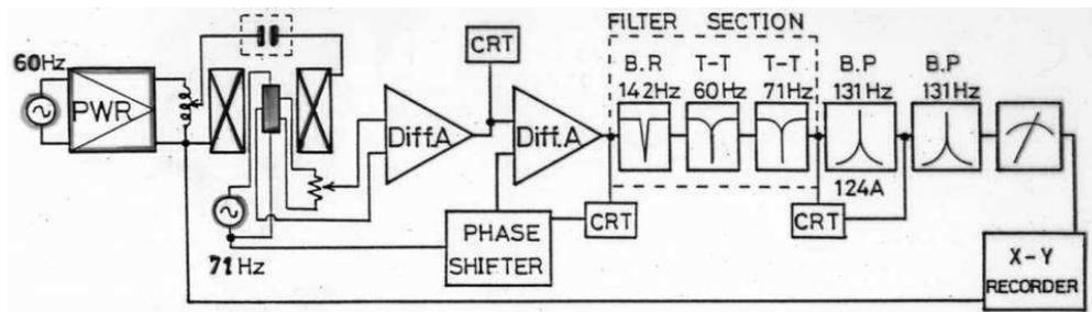
Fig. 1. Diagram of the two-frequency ac method.
