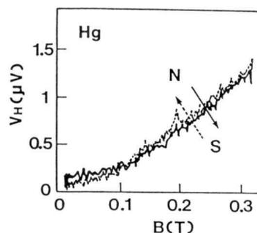
Fig. 6. Hall signal in liquid state of Hg through ac-dc method.
