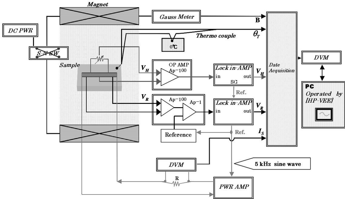
Fig. 10. Block diagram of measurement circuit.
