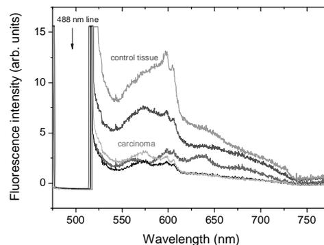
Fig. 4. AF spectra collected from normal and malignant part of colon tissue are shown. Spectra were single fibre collected and detected by Avantes spectrometer.
