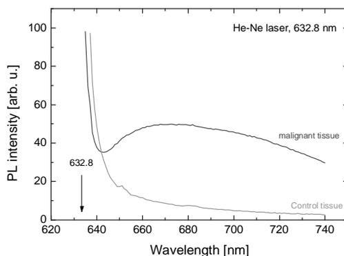
Fig. 1. Fluorescence spectra of human colon tissue taken at room temperature and excited by He-Ne laser at the power density of 200  $\text{mW}/\text{cm}^2$ . The arrow indicates the wavelength 632.8 nm of the exciting laser. In the case of control sample (normal tissue) only the tail of scattered laser signal is detected; there is no luminescence from the sample. In the case of malignant tissue we can see a broad luminescence curve centred around 670 nm.
