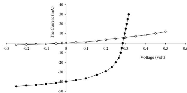
Fig. 7. I – V characteristic of CuInSe<sub>2</sub>/CdTe solar cell in dark and illumination at room temperature.
