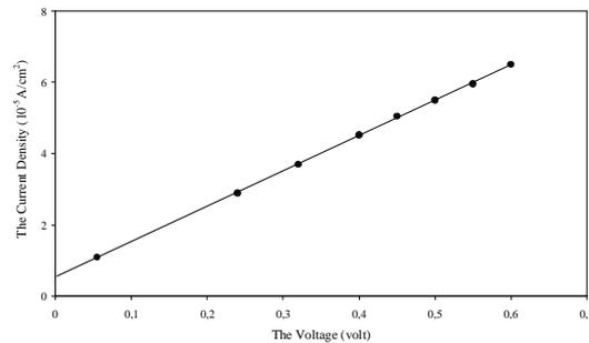
Fig. 5. Relation of current - voltage characteristic of CuInSe<sub>2</sub>/CdTe solar cell due to the series resistance in dark condition.
