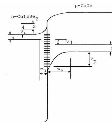
Fig. 6. Energy band diagrams of CuInSe<sub>2</sub>/CdTe solar cell.
