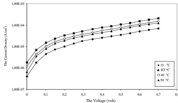
Fig. 3. Semilogarithmic relation of current voltage characteristic of CuInSe<sub>2</sub>/CdTe heterojunction cell in dark condition at different temperatures.
