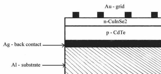
Fig. 1. Schematic diagram of a cross-section of  $\text{n-CuInSe}_2/\text{p-CdTe}$  solar cell.
