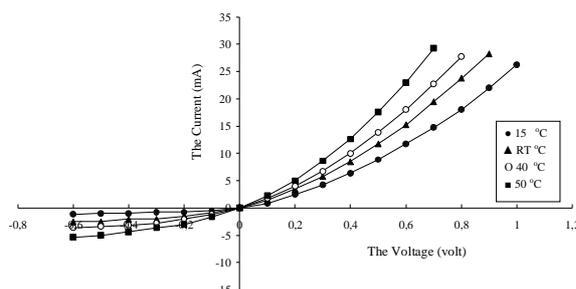
Fig. 2. I – V characteristics of  $\text{CuInSe}_2/\text{CdTe}$  heterojunction in dark condition at different temperatures.
