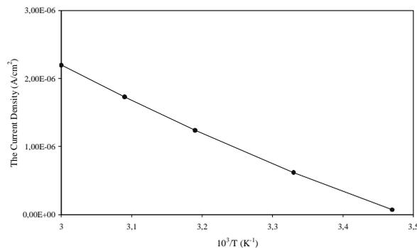
Fig. 4. The current density versus  $1/T$  of CuInSe<sub>2</sub>/CdTe heterojunction solar cell in dark condition.
