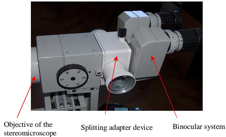
Fig. 3. The splitting device connected to the Fotobioftal-1.
