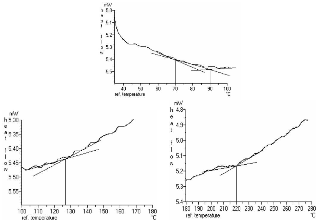
Fig. 4. The DSC thermogram of undoped Ultem film divided to three temperature ranges.
