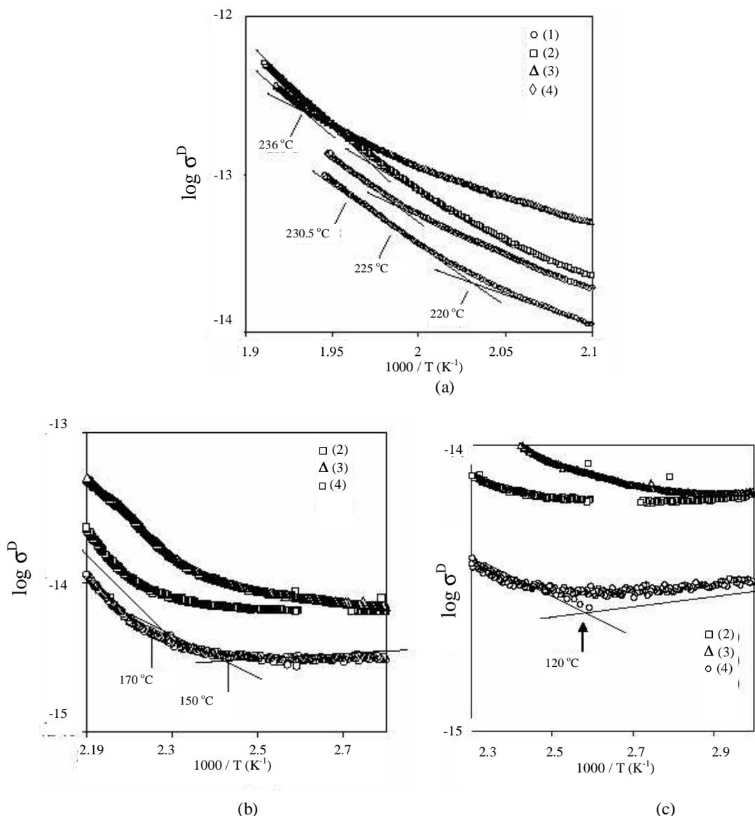
Fig. 3. Arrhenius plot of the conductivity of Ultem film: undoped (4), 0.25 mol/mol polymer (1), 0.5 mol/mol polymer (2) and 0.75 mol/mol polymer (3) doping ratio at different temperature ranges.
