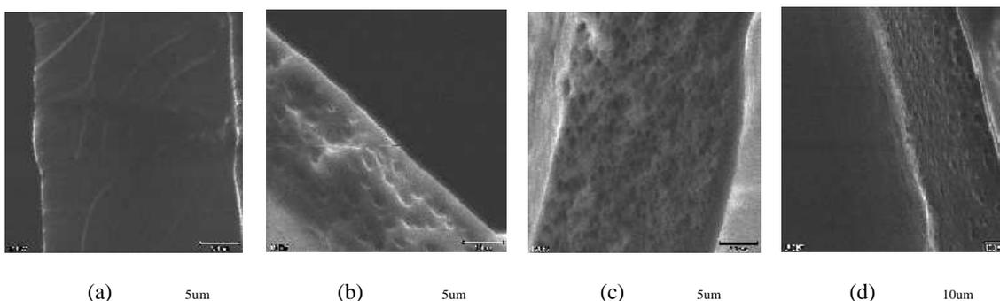
Fig. 4. SEM pictures of undoped (a) and doped Ultem films with the dopant concentration of 0.25 mol (b), 0.50 mol (c) and 0.75 mol (d) per mol of polymer.
