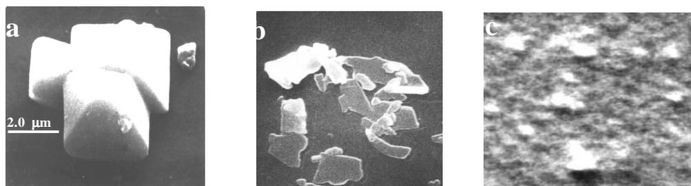
Fig. 1. SEM micrographs (a,b) of 100 nm thick  $\text{As}_2\text{S}_3$  (a) and  $\text{GeSe}_3$  (b) films after heavy UV irradiation. Optical micrograph of photolytic Ag (black) in 400 nm thick AgBr film (c).
