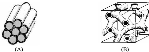
Fig. 2. Pore structure of molecular sites type A) SBA-15; B) MCM-48.
