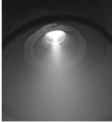
Fig. 2. The visual aspect of the discharge in the sputtering regime.
