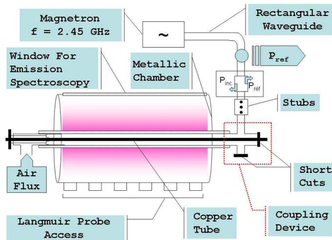
Fig. 1. Longitudinal cut of the experimental set up.
