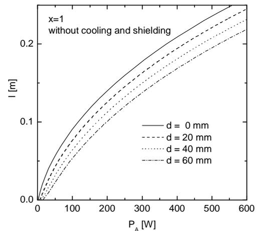
Fig. 7. Dependence of a single plasma column length on  $P_A$ , for different values of  $d$ .
