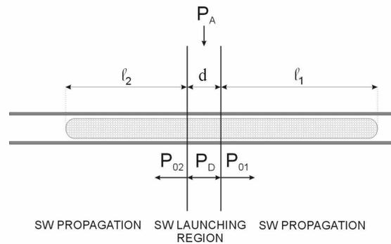
Fig. 5. Axial structure of a SWD.
