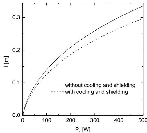
Fig. 4. Dependence of plasma column length on wave power for two cases: discharge tube is surrounded by cooling liquid and shielding grid – dotted line; discharge tube is surrounded by air – solid line.
