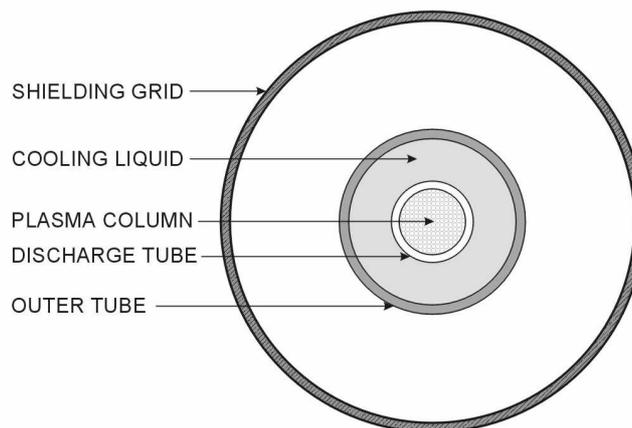
Fig. 1. Cross-section of the discharge setup.
