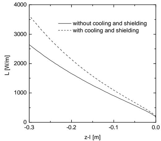
Fig. 3. Axial distribution of  $L$  for two cases: discharge tube is surrounded by cooling liquid and shielding grid – dotted line; discharge tube is surrounded by air – solid line.
