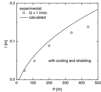
Fig. 10. The plasma column length vs absorbed power for case with cooling and shielding.
