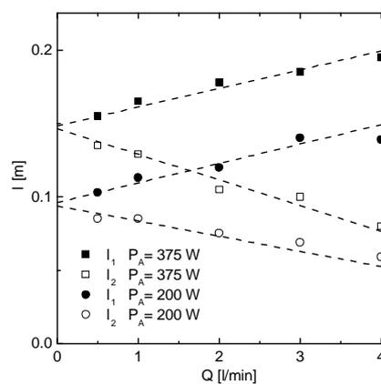
Fig. 8. Experimental values of column length vs intensity of gas flow for two values of absorbed power.
