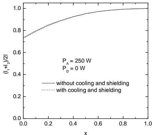
Fig. 6. Dependence of sum of plasma column lengths on  $x = l_2/l_1$ , for two cases: discharge tube is surrounded or not by cooling liquid and shielding grid.
