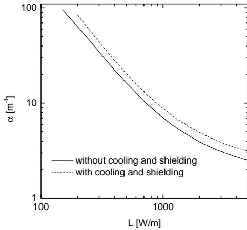
Fig. 2. Dependence of attenuation coefficient  $\alpha$  on  $L$  for two cases: discharge tube is surrounded by cooling liquid and shielding grid – dotted line; discharge tube is surrounded by air – solid line.
