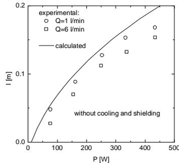
Fig. 9. The plasma column length vs absorbed power for case without cooling and shielding.
