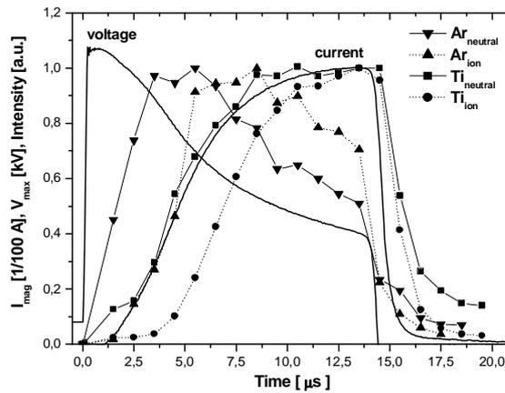
Fig. 2. Time dependences of the magnetron current, voltage and lines intensities taken from the magnetron area at distance 1.2 cm from target.
