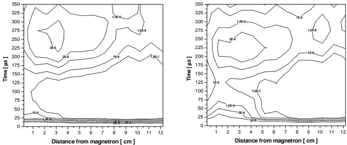
Fig. 4. Time and spatial evolution of Ti (left) and  $Ti^+$  (right) intensities in magnetron-substrate holder area. At the distance of 10 cm, the density of electrons created by the microwaves is maximal.
