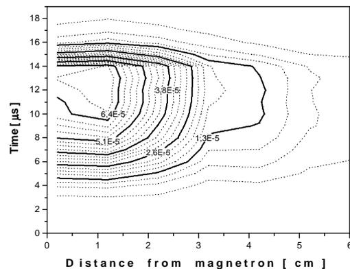
Fig. 3b. Time and space distribution of  $\text{Ti}^+$  line intensity near the target during the pulse.
