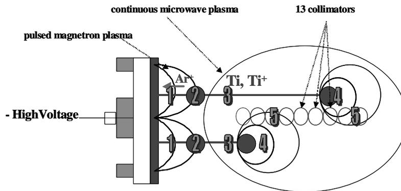
Fig. 5. Schematic representation of the relevant processes concerning the creation and transport of the species in the pulsed magnetron discharges.
