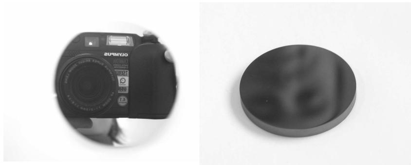
Fig. 6. Photos of a 10.1 micron thick EV-TAS1 film deposited on a  $\text{As}_2\text{S}_3$  commercial target of 5 cm in diameter and further polished down to 0.2 micron.
