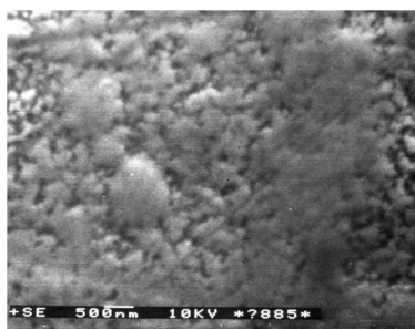
Fig. 1. Scanning electron microscopy of the sample (A) showing the multinuclear growth of the films. The marker bar shown in the image has a dimension of 500 nm.
