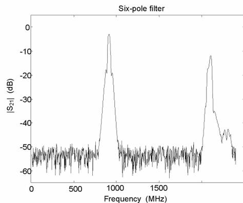
Fig. 14. The measured frequency response of the six-pole GSM / GPRS filter.
