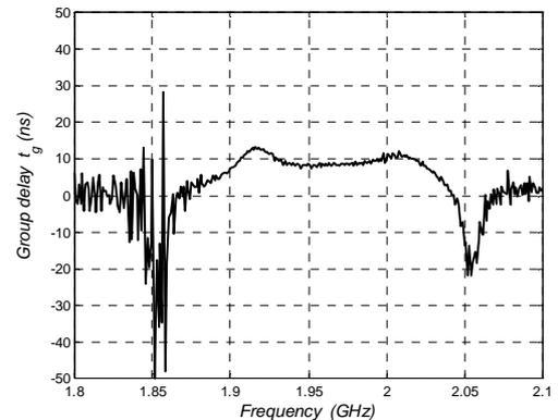
Fig. 4. Measured group delay of the first filter model shown in Fig. 2.
