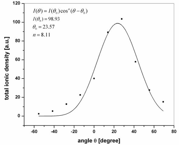
Fig. 4. Angular distribution of the maximum ionic current. The solid line is the fit of experimental data to Eq. (1).
