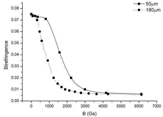
Fig. 2. Magnetic field dependence of birefringence, for two LC cells with planar alignment.
