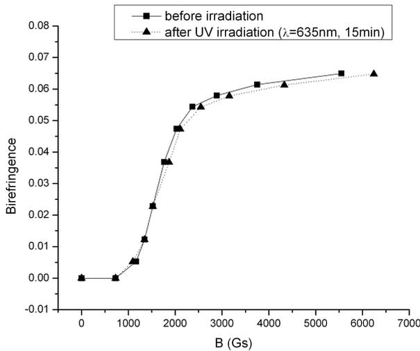
Fig. 3. Magnetic field dependence of birefringence, for a LC cell ( $d = 180 \mu\text{m}$ ) with homeotropic alignment, before and after UV irradiation.
