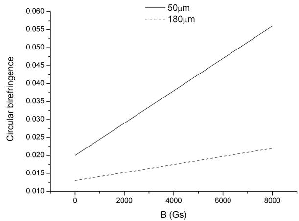
Fig. 4. Magnetic field dependence of circular birefringence, for planar aligned LC cells with two different thicknesses.
