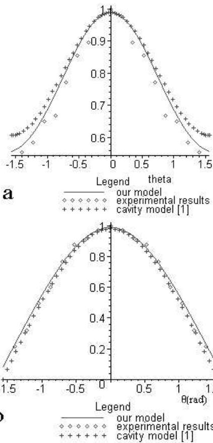
Fig. 3. Radiation pattern for a 3 GHz antenna: a-  $\phi = 0^\circ$  plane; b-  $\phi = 90^\circ$  plane.
