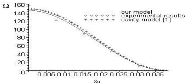
Fig. 4. Impedance dependence with the feeding point for a 1.187 GHz patch.
