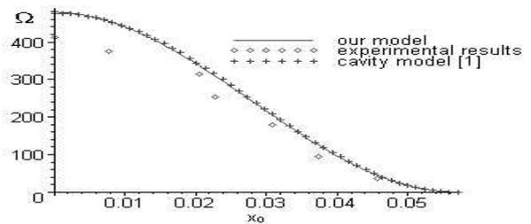
Fig. 6. Impedance dependence with the feeding point for a 803 MHz patch.
