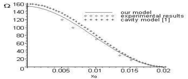
Fig. 5. Impedance dependence with the feeding point for a 2.3 GHz patch.
