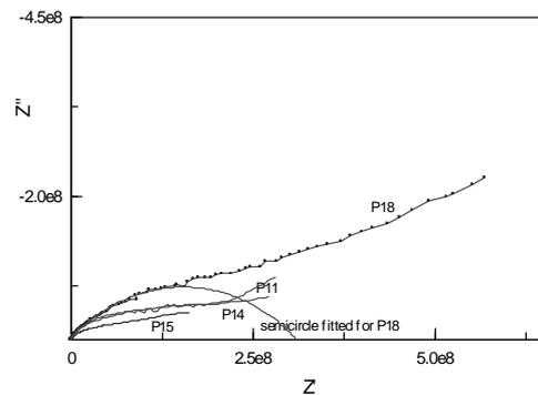
Fig. 5. Cole - Cole plot for the samples with constant graphite content (10%) and various the ratio of kaolin/alumina (P11 85/15, P14 70/20, P15 65/25, P18 50/40).
