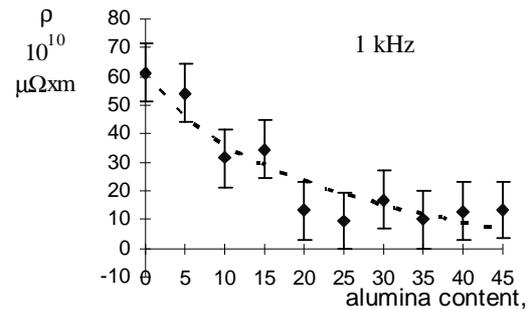
Fig. 1. The influence of alumina/kaolin ratio on electrical resistivity at fixed graphite content, 10%.
