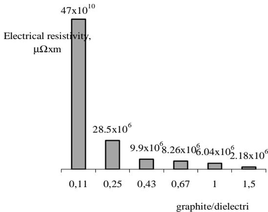
Fig. 2. The evolution of electrical resistivity as a function of conductive/dielectric phase ratio.
