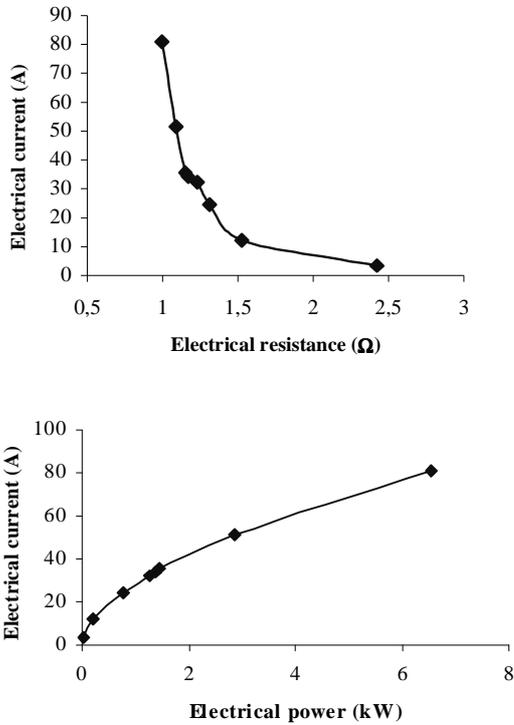
Fig. 12. Electrical characteristics for a stack of three resistors. Each resistor has the same size: diameter is 80 mm and thickness 10 mm.
