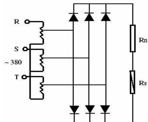
Fig. 11. Electrical diagram for measuring a three stack resistor  $R_n$ , using a bridge.
