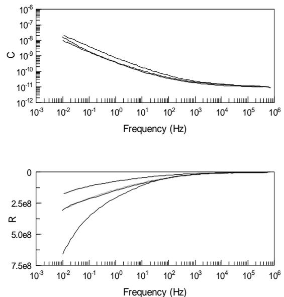
Fig. 7. Comparative frequency response in the range  $10^{-2}$  –  $10^6$  Hz of the composite pellets at room temperature ( $\sim 25^\circ\text{C}$ ), in the approximation of composites representation as RC parallel circuits. C = Capacity and R = Resistance.
