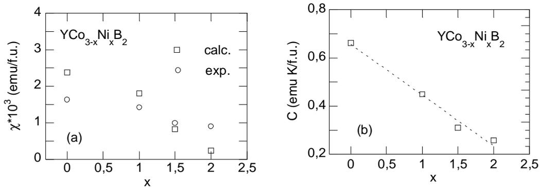
Fig. 2. Composition dependencies of the magnetic susceptibilities at 4.2(2) K experimentally determined and obtained from band structure calculations (a), and of the Curie constants (b) in  $\text{YCo}_{3-x}\text{Ni}_x\text{B}_2$  compounds.
