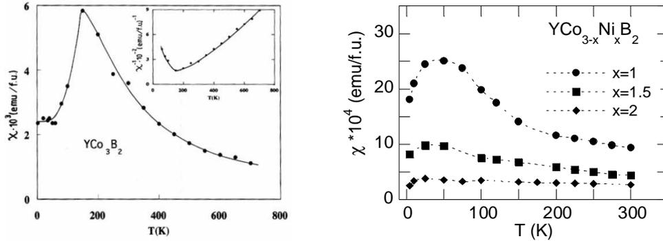
Fig. 1. Thermal variations of magnetic susceptibilities for  $\text{YCo}_{3-x}\text{Ni}_x\text{B}_2$  compounds.
