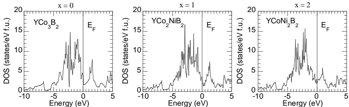
Fig. 3. DOS for  $\text{YCo}_{3-x}\text{Ni}_x\text{B}_2$  compounds with  $x=0, 1$  and  $2$ .
